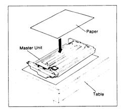
3. To protect the master surface, put the master unit on a flat table and put a sheet of paper on the master unit.
